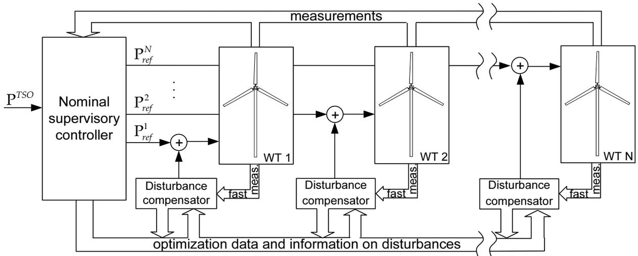
Figure 1: Wind farm hierarchical control system
